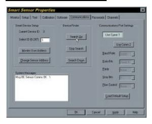
There are many different computers capable of using this software, so LTH have built in the ability to tweak the basic serial data settings if you wish to do so.
