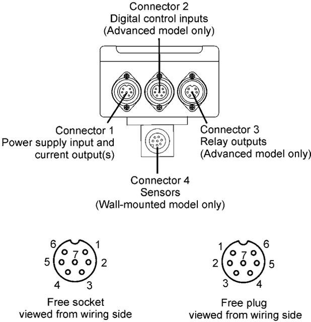
Figure 4 Wall mount unit, rear view
