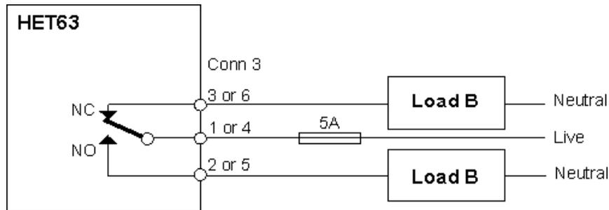
Figure 5 : Relay contact connection
