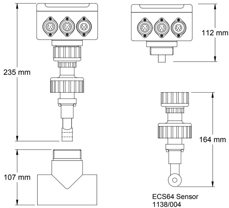
Figure 1 Head-mounting Installation components
