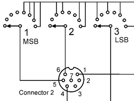
Figure 7 : Rotary switch connections
