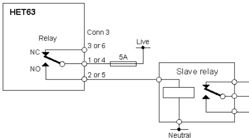
Figure 6 : Slave relay connection
