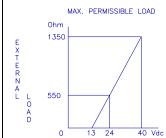
The maximum permissible load(Ri max.) in case of 24 Vacis 550 Ù (Ohm).
