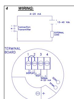
The connector, and **zero** / **span** potentiometers are under the cover. Testnipples for calibration of the SERIES 8000 and SERIES 8000-SAN are available on request.
