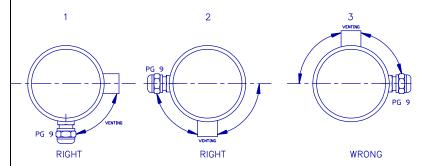
When the transmitter is mounted horizontal, the venting MUST be pointed horizontal to downwards. See figure left.
