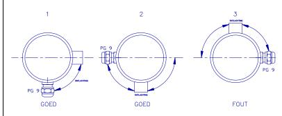
When the transmitter is mounted horizontal, the venting MUST be pointed horizontal to downwards. See figure left.
