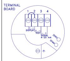
The connector, and **zero** / **span** potentiometers are under the cover. Testnipples for calibration of the SERIES 8000-RANGE-VALVE are available on request.
