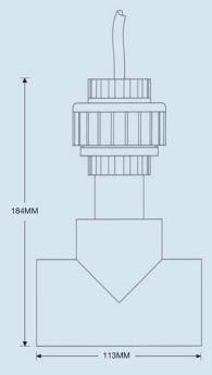
S400 1.5" Quick release PVC tee assembly for inline mounting of the S400 electrodes.
