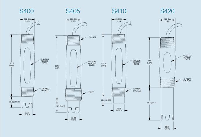
The S400 sensors have been designed for rugged service in submersion or inline process applications. The reference cell features a double junction design for extended service life in harsh applications. The high quality sensors are constructed of corrosion resistant wetted materials including Ryton®, Teflon® and glass. They can be supplied with built in temperature compensation and a solution ground connection.
