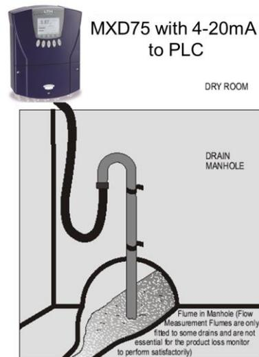
Because of Quadbeam's ratio-metric four beam method of measurement the instrument effectively self-compensates for variation in temperature and fouling of the fingers, providing an accurate and repeatable signal. The LTH MXD70 Series transmitters can take up to three sensors where there are multiple drains and can accept other measurements such as Turbidity, Conductivity, pH/ORP & Dissolved Oxygen sensors in any combination.
