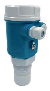
Flowmeter is an ultrasonic flow transmitter, temperature-compensated and suitable for connection with MODBUS RTU acquisition systems. FLOWMETER in addition to an analog output includes two freely addressable relay for flow threshold or for totalizer pulse output.
