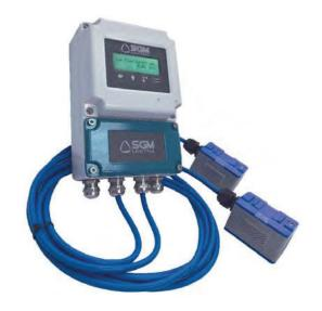
The SGM-101F flowmeters operate on the ultrasonic pulses transit time difference principle. The great advantage is the mechanical installation, because it is not necessary to cut the pipe. The sensors are simply clamped on the outer pipe surface, for this reason the pressure and the liquid aggressiveness to be measured are not a problem for the fl owmeter. The system measures in a bidirectional way and is suitable for clean or slightly dirty liquids.
