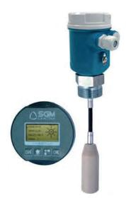
CLS5 is a capacitive level control instrument that uses an advanced technology. CLS5 is equipped with a sensor in PP heat-sealed. This allows its use in a wide applications range for the level control in granules or powders such as cement, flour, feed for animals, etc. .. The CLS5 is easily configurable via the VL601 module. Maximum tensile load 3000 N.
